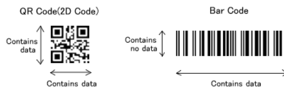
FIGURE I. Comparison of QR code and Bar code [3].
